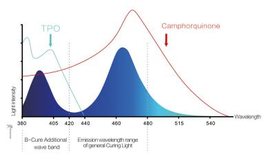
The light-absorbing peak of traditional material (including camphorquinone; the red line on the figure) is 460nm, so the curing can be done by either general Curing Light or Wide Spectrum Curing Light.
