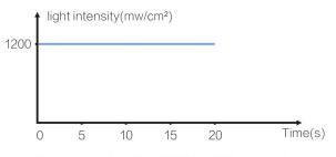
Constant intensity of 1000-1200 mw/cm²; Time setting: 5s, 10s, 15s and 20s.
