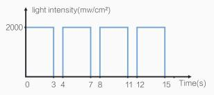
10 cycles with an interval of 1s after each cycle; Time setting for each cycle can be 3s or 5s.
