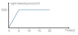
Light intensity increases from 0 mw/cm<sup>2</sup> to 1200 mw/cm<sup>2</sup> in 5 sec. Time setting: 5s, 10s, 15s and 20s.
